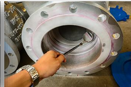
Dye Penetrant Testing
